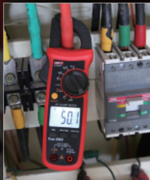
High voltage (600V) frequency measurement
