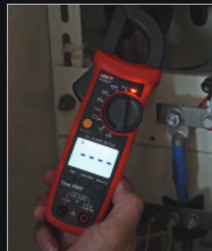
NCV multi-segment display and audio/visual alarm
